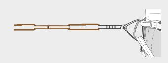
To attach the Multi Chain to the harness use only the special knot which is now explained: thread the bottom loop of the daisy chain through both harness loops as shown and pass it through the tie-in loop; thread the top loop through the bottom loop and pull it away from the body until the knot is tight. Check the knot is correctly tied. Using the special knot the breaking strength of the Multi Chain remains equal to 24 kN.
